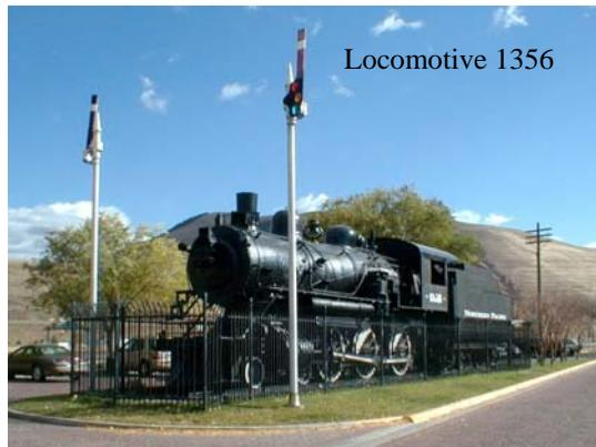
This project included removal of all asbestos associated with the boiler and brake system, repair and replacement of woodwork, and painting of this historic train engine donated to the City in 1955.
