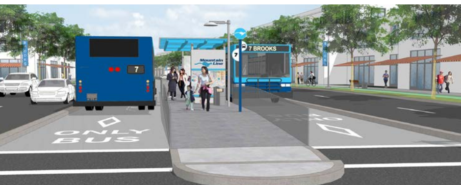
A fixed, center-running transit guideway improves transit travel times and transit reliability, and signals permanence to developers. Center transit stations provide refuge points for pedestrians crossing Brooks Street, and can also become focal points on the corridor.
