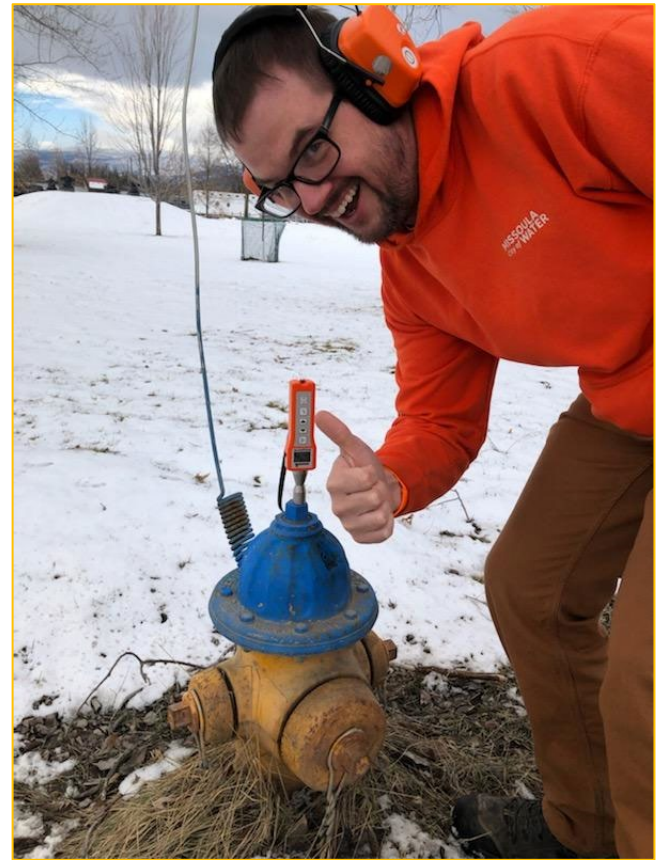
Leak detection equipment helps us find water main leaks.
