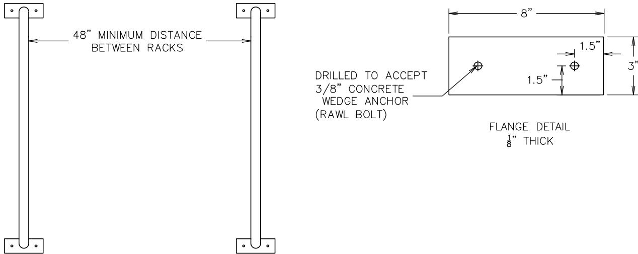
WELDING SHALL BE 100% AND WELDED WITH  $\frac{1}{4}$ " FILLET WELDS.
