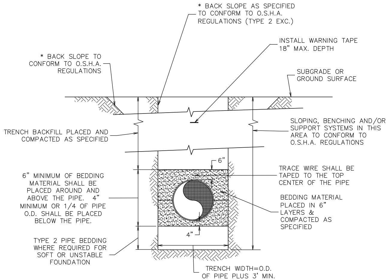
\* SEE O.S.H.A. CONSTRUCTION STANDARDS FOR EXCAVATIONS, SECTION 1926, SUBPART P.
