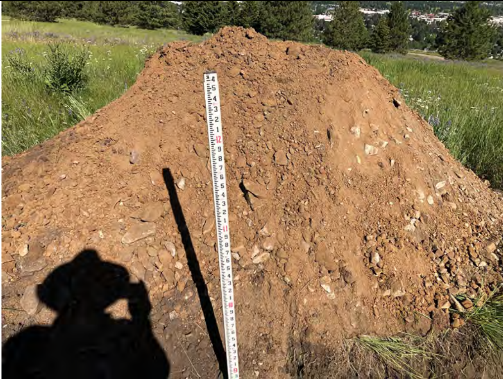
Description: TP-20 Spoils pile from above 7.5 feet.
