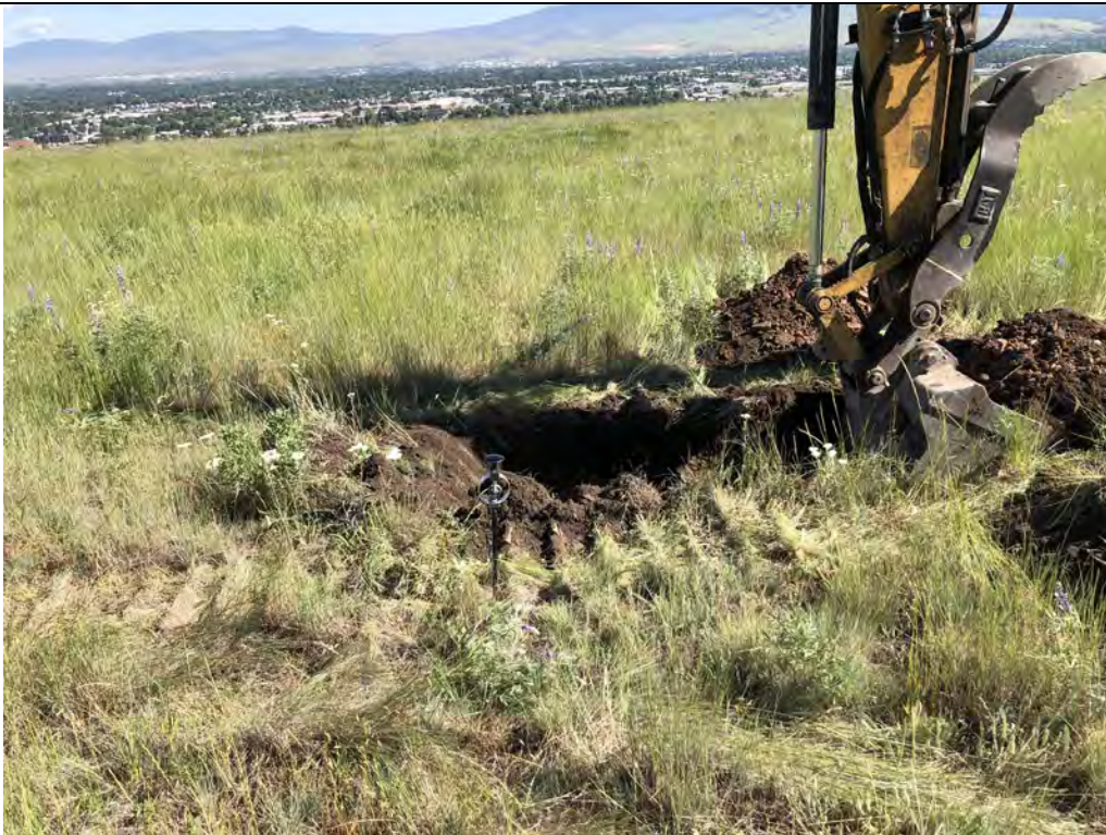
Description: TP-19 Location. View is to the north. Cone penetrometer was pushed 7.25 inches under a 320 psi loading.
