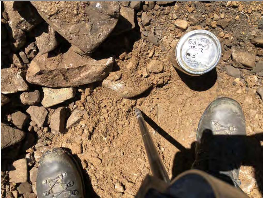
Description: TP-12 Jar sample from 3 feet. Cone penetrometer was pushed 2 inches under a 320 psi loading.
