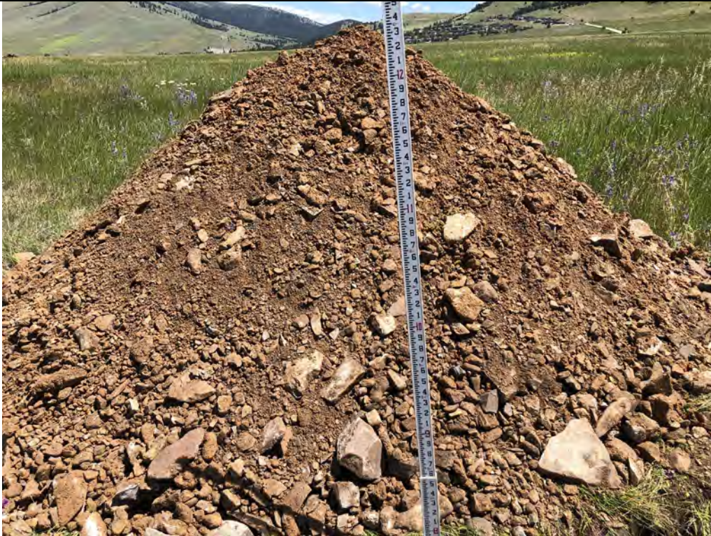
Description: TP-12 Spoils pile from above 8 feet.
