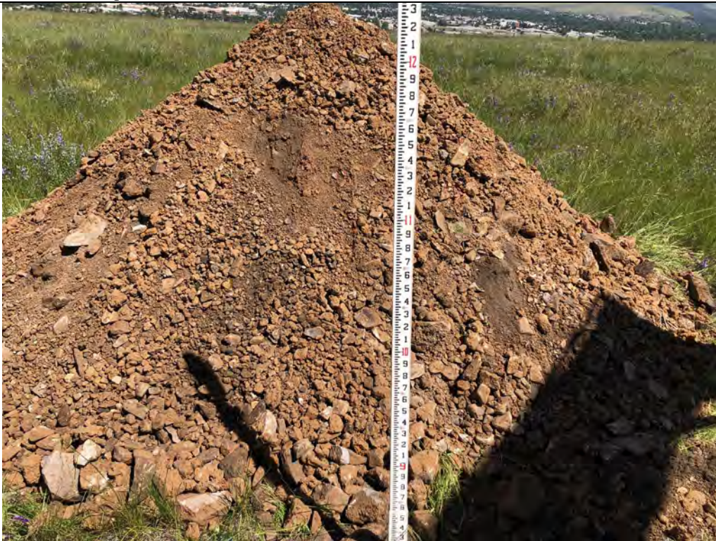
Description: TP-19 Spoils pile from above 8.25 feet.
