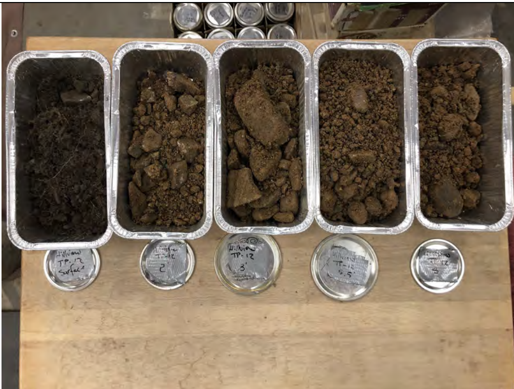
Description: TP-12 Moisture content samples prior to being placed into the drying oven.
