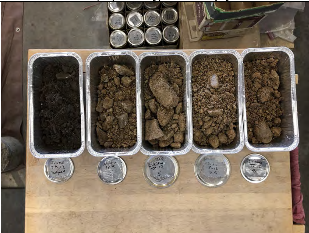
Description: TP-12 Moisture content samples after being taken out of the drying oven.
