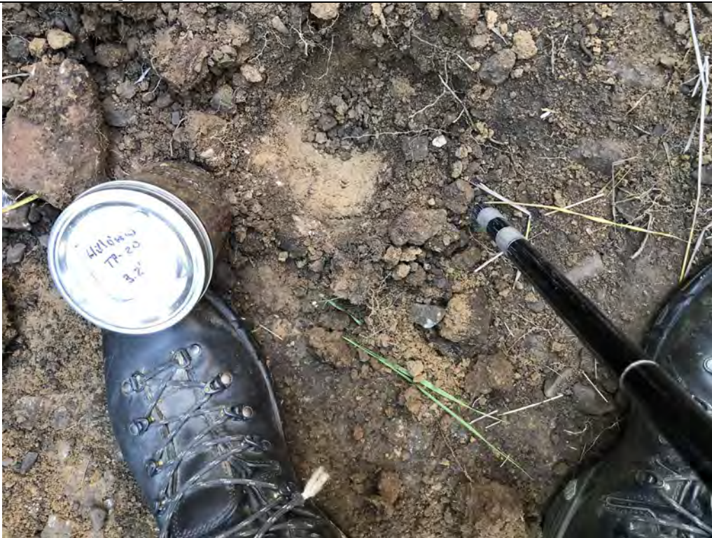
Description: TP-20 Jar sample from 3.2 feet. Cone penetrometer was pushed 3.5 inches under a 320 psi loading.
