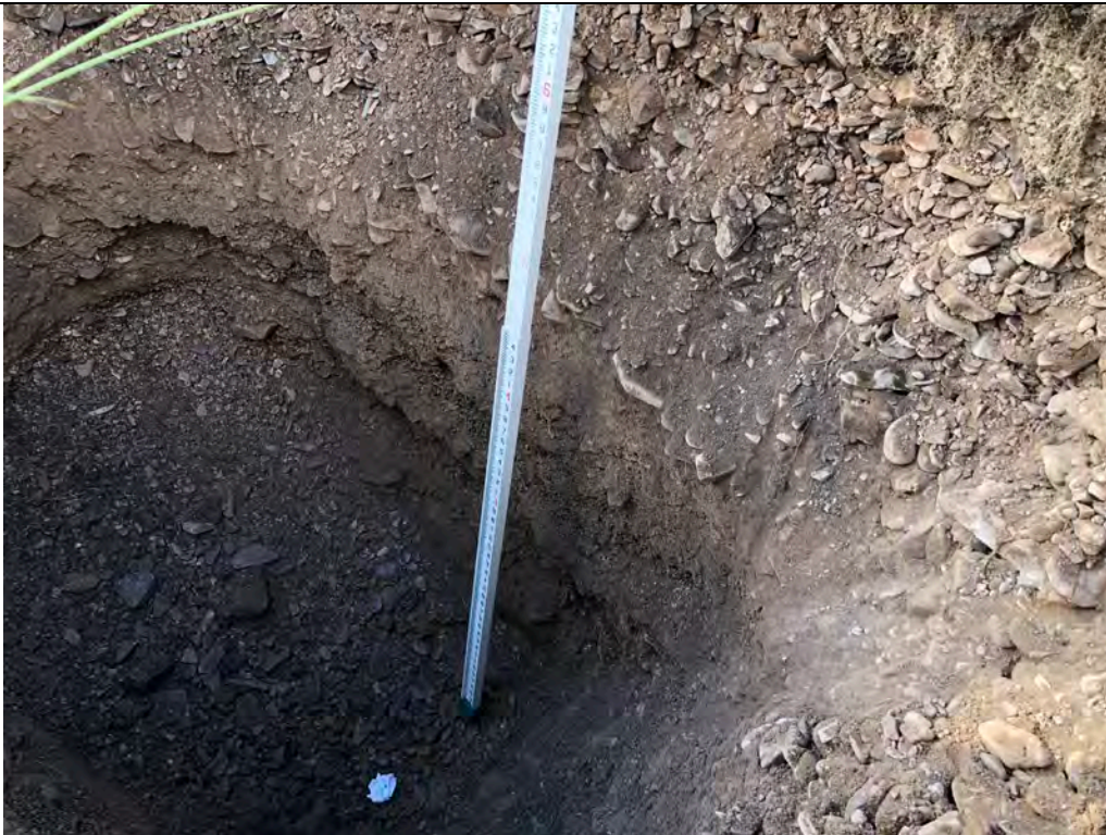
Description: TP-15 Excavated to 8 feet.
