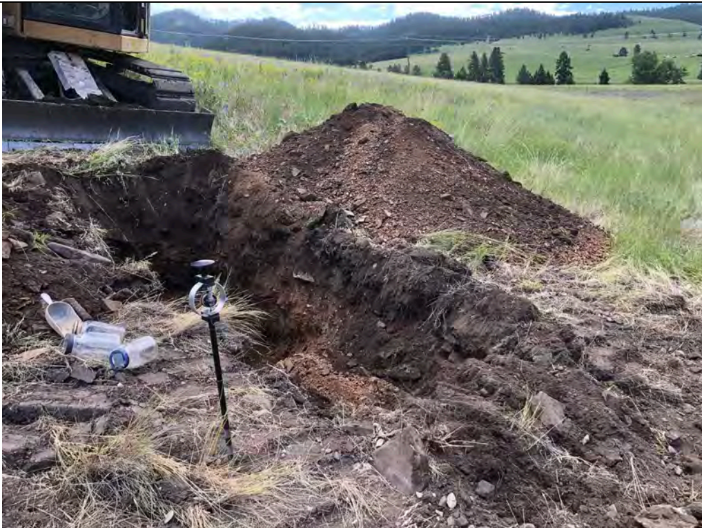
Description: TP-10 Army Corps of Engineers Cone Penetrometer was pushed 2.75 inches under a 320 psi loading. View is to the southeast.
