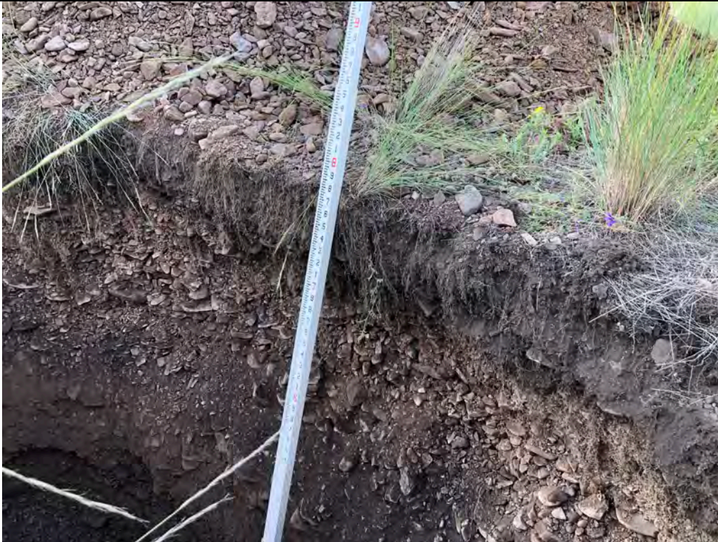
Description: TP-15 Excavated to 8 feet.
