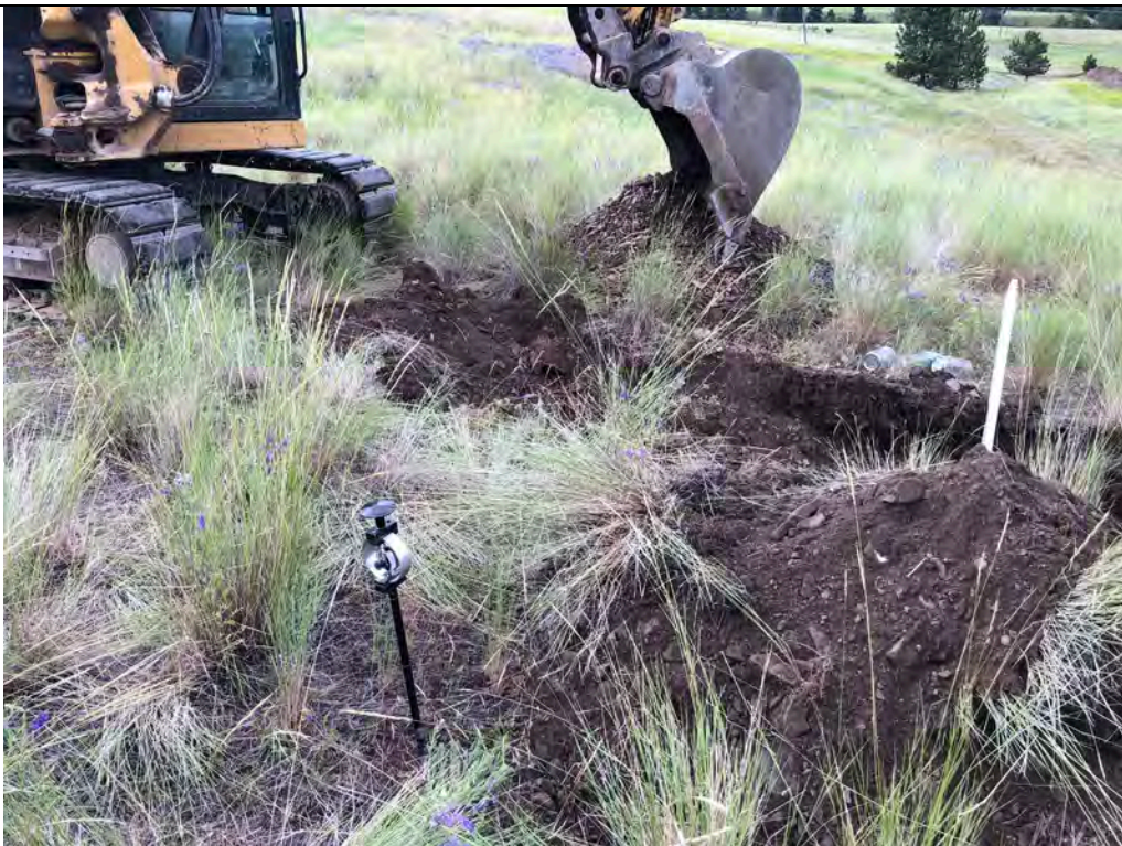
Description: TP-15 Cone penetrometer was pushed 4.25 inches under a 320 psi loading. View is to the south.
