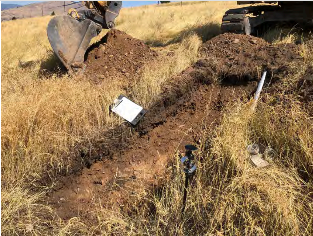
Description: TP-10 Location. Cone penetrometer was pushed 0.5 inches under a 320 psi loading. View is to the east.
