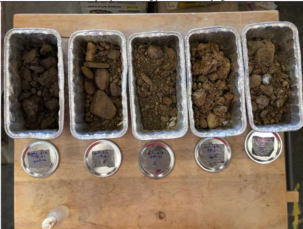
Description: TP-01 Moisture content samples after being taken out of the drying oven.
