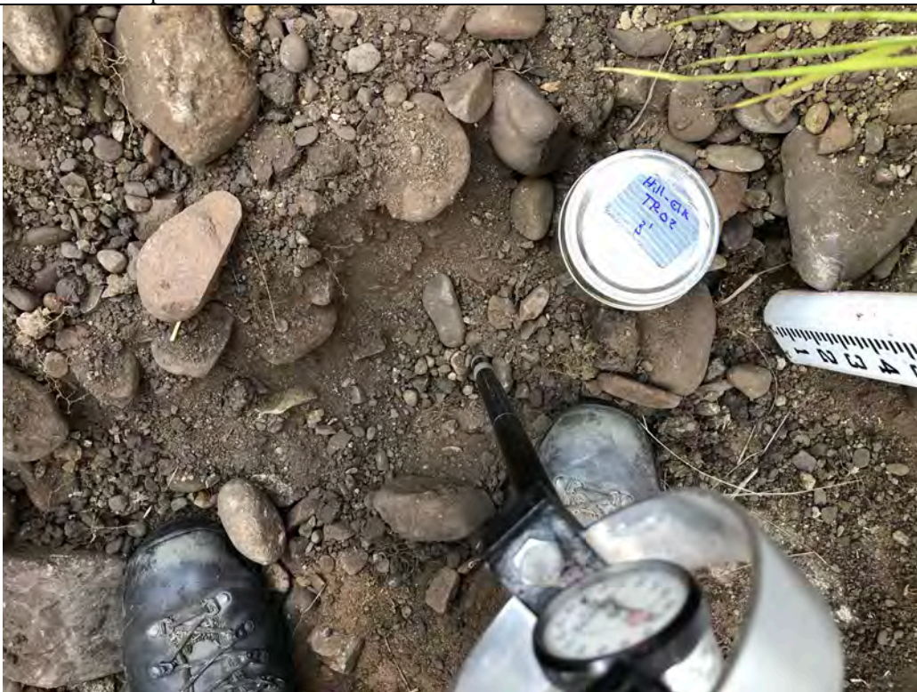
Description: TP-02 Jar sample from 3 feet. Cone penetrometer was pushed XX inches under a 320 psi loading.
