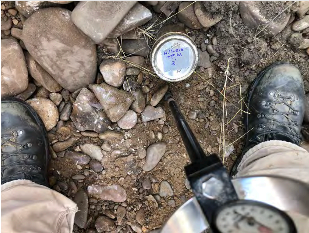
Description: TP-01 Jar sample from 3 feet. Army Corps of Engineers Cone Penetrometer was pushed XX inched under a 320 psi loading.
